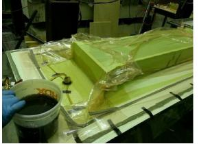
(e) VARTM Process (f) Final Deck after Demolding Figure 3.2 Construction Stages of Hybrid System
