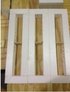
Figure 3.24 Specimen Preparation Showing the Plywood Position
