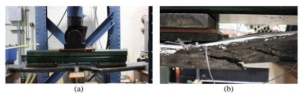
Figure 4.26 Failure Mode of Specimen 1T2S: (a) Deflected Shape, and (b) Shear Crack
