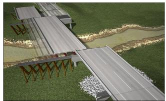
Figure 2.12 Rendering of Bridge Spans Laterally Sliding into Place
