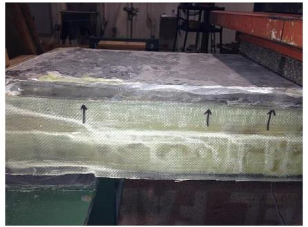
Figure 3.14 The Failure Mode near the End of the Grouted Region
