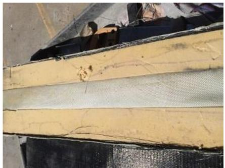
Figure 3.11 The FRP Cloth after Demolding
