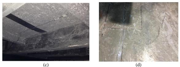
Figure 4.34 Flexure Test and Failure Mode of Specimens 4T1S-HSS, (a) Test Setup, (b) Beam Shear Crack, (c) Cracks on the Slab, and (d) Cracks on the Top Slab
