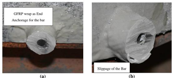
Figure 4.16 Simple End Anchorage System for CFRP Bars in Phase 1: (a) Grinded End, and (b) Slippage of CFRP Bar
