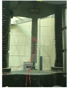
Figure 3.33 Double Lap Specimen Arrangement during the Test
