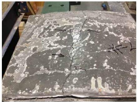
Figure 3.12 Failure Mode near the End of the Grouted Region
