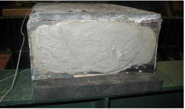
Figure 3.9 End of the Specimen after Grouting
