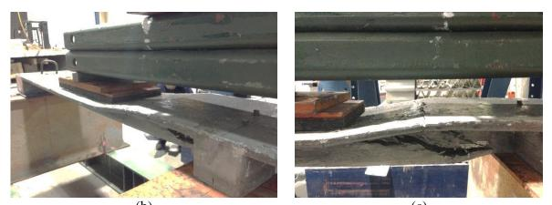
(b) (c) Figure 4.43 Flexure Tests of Specimen 1T2S-HSS: (a) Test Setup, (b) Deflected Shape, and (c) Failure Mode
