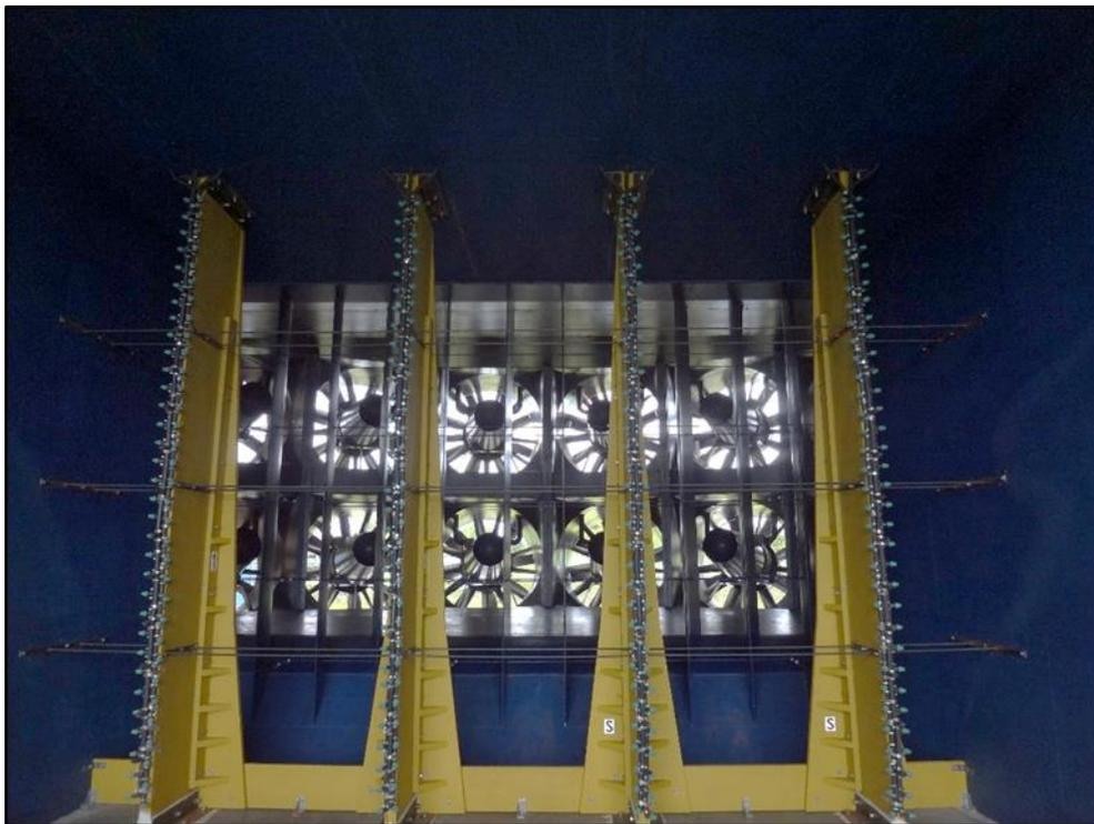
Figure 3.20 Wind driven rain test nozzle configuration
