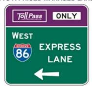
Figure 2-2: Examples of Guide Signs before Entrances to Priced Managed Lanes (Source: FHWA, 2009)
