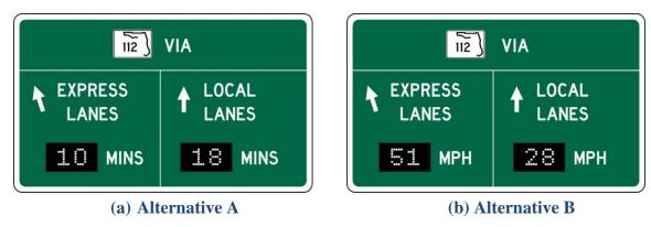
Figure 4-9: Sign Alternatives Displaying Travel Times and Average Travel Speeds on Express Lanes and General-purpose Lanes
