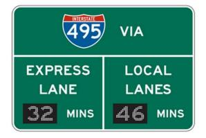
Figure 2-3: Example of a Comparative Travel Time Information Sign for Preferential or Managed Lanes (Source: FHWA, 2009)
