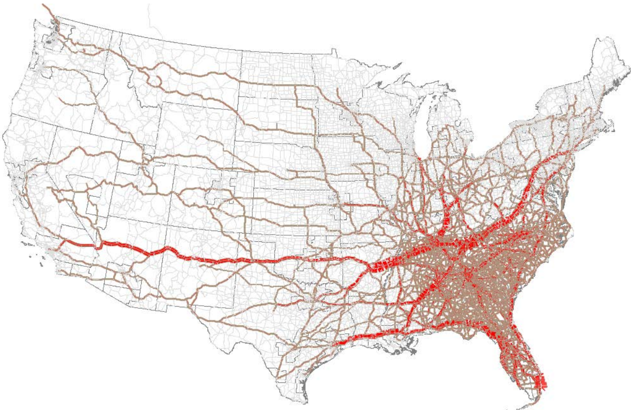
Figure 2.4 Truck Flows between O-D Pairs that influenced I-85 Corridor Traffic in 2007 (estimated, based on FAF3 and other data sources)
