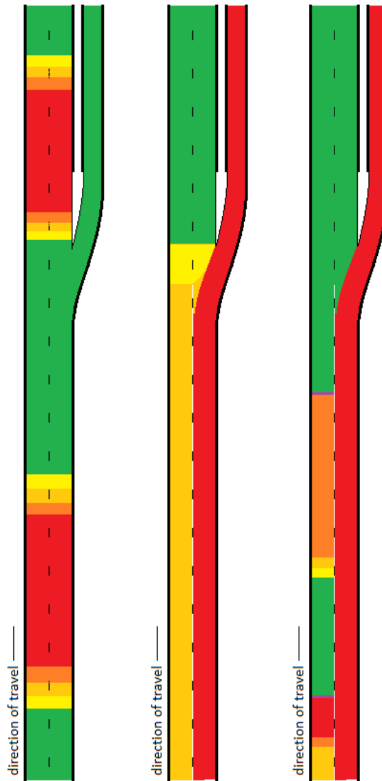
a. Wave Propagation b. Friction Factor c. Lane Changing Disruption
