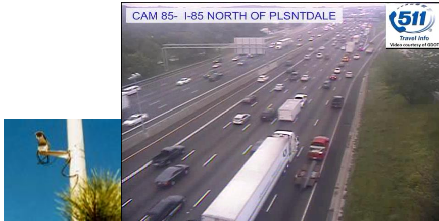
Figure 11: PTZ Camera and General View
