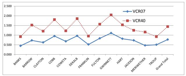
Figure 1.5 2007 and 2040 Volume/Capacity Ratios (VCRs) along I-85/I-285, by County (Source: Derived from FAF3 estimates).
