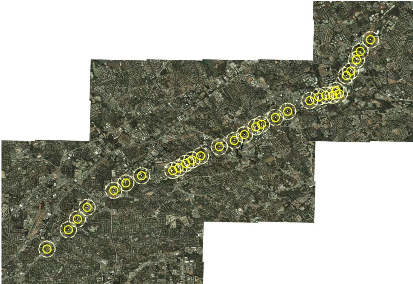
Figure 4: Camera Coverage on I-85 Corridor
