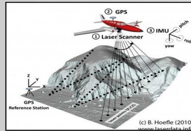
purpose of this investigation is to identify methods capable of identifying sinkholes near vehicular roadways. Research shows that the airborne laser mechanism is the most capable at detecting a potential sinkhole, because of the ability to compute a displacement in angle of the laser during flight.
