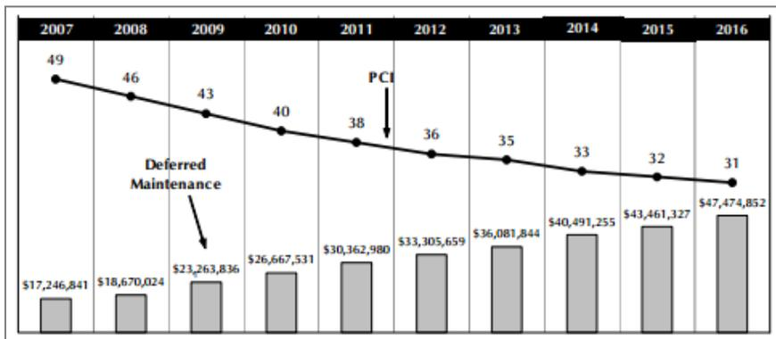
Figure 3: Current Service Level Road Condition and Backlog (1)
