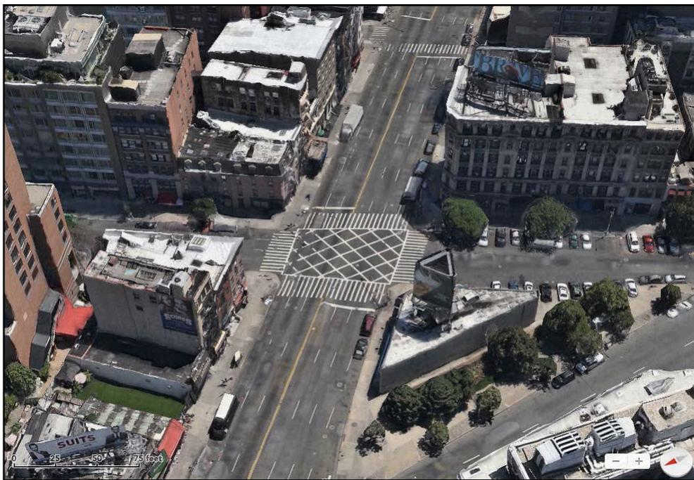
**Figure 4: Box Junction on Canal Street in Manhattan (27).**
