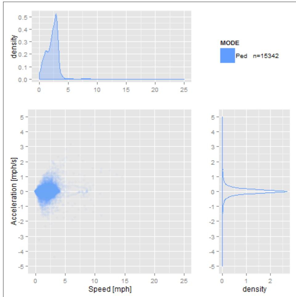
**Figure 36. Pedestrian Speed and Acceleration**
