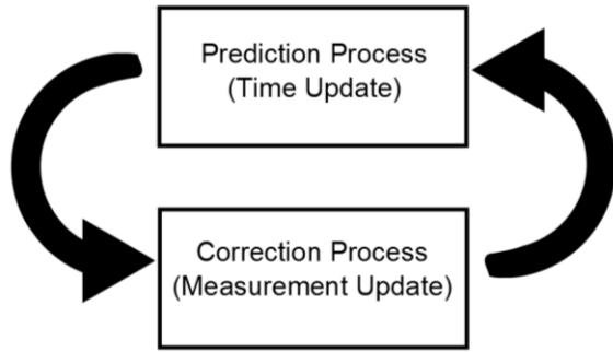
**Figure 15. The Kalman Filter Cycle**
