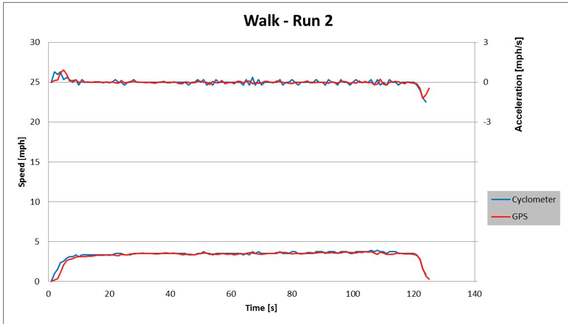
**Figure 58. Lab Test Speed and Acceleration – Walk 2**
