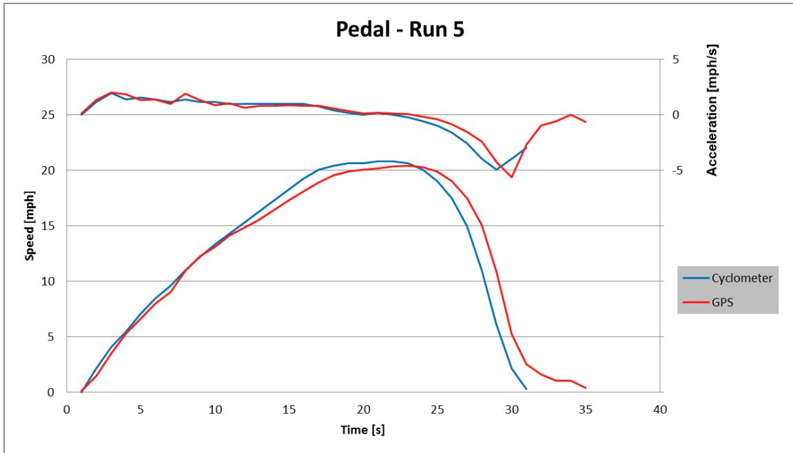
**Figure 81. Lab Test Speed and Acceleration – Pedal 5**
