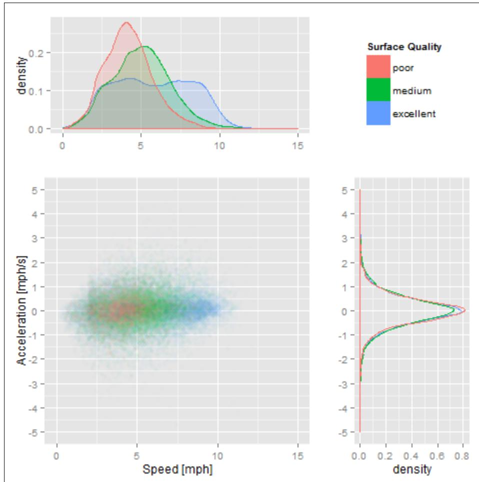
**Figure 45. Effect of Surface Quality on Segway Speed and Acceleration**
