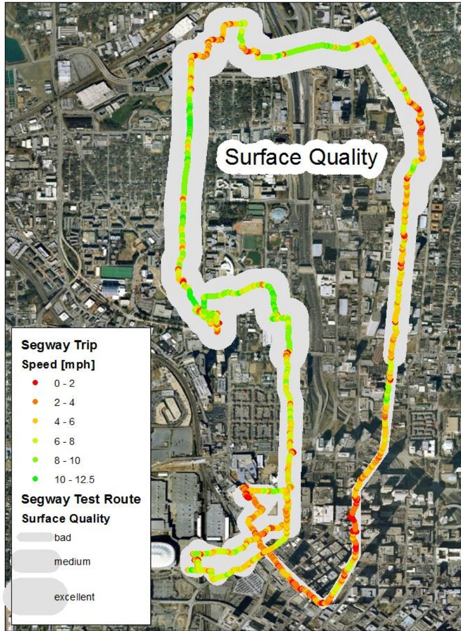
Figure 44. Map of Segway Test Trip Speed by Surface Quality
