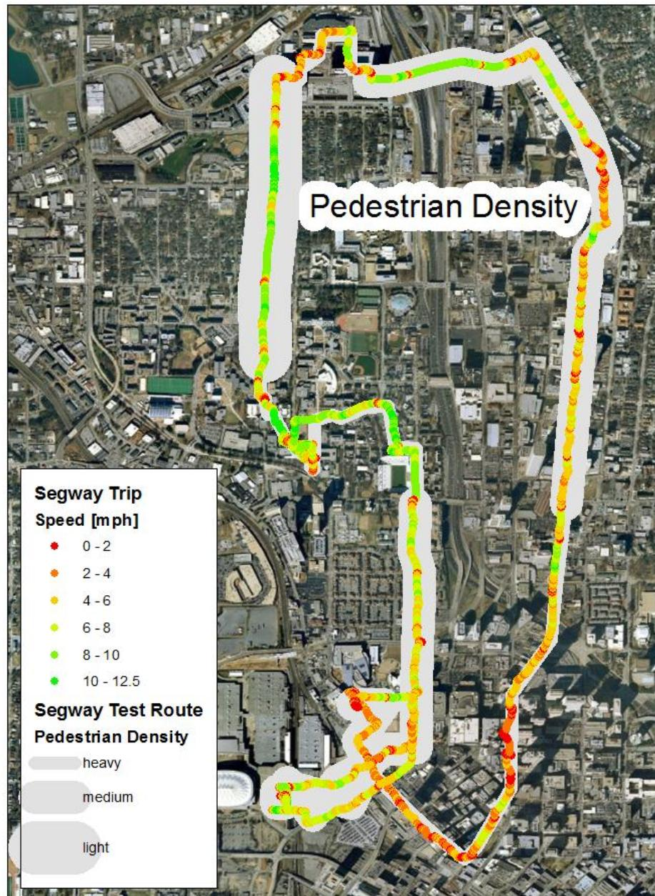
Figure 46. Map of Segway Test Trip Speed by Pedestrian Density
