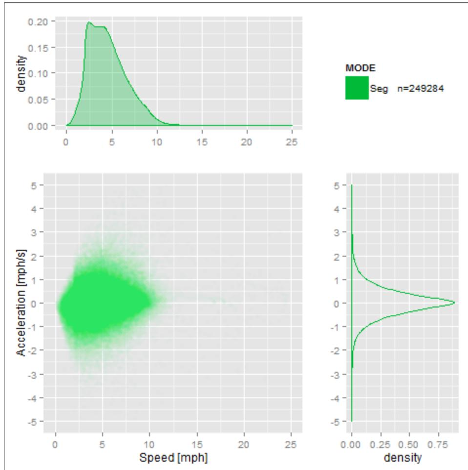
**Figure 37. Segway Speed and Acceleration**
