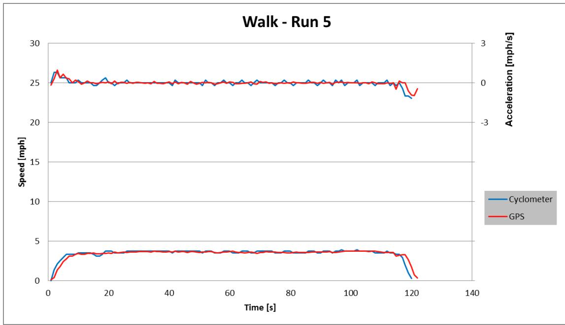
**Figure 61. Lab Test Speed and Acceleration – Walk 5**
