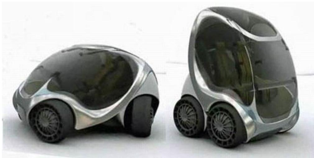
**Figure 7. MIT CityCar in Both Driving (left) and Parked (right) Configurations**
