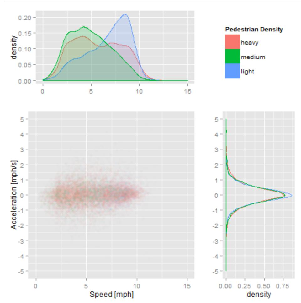
**Figure 48. Segway Test Speed and Acceleration by Pedestrian Density on Wide Sidewalk with Excellent Surface Quality**
