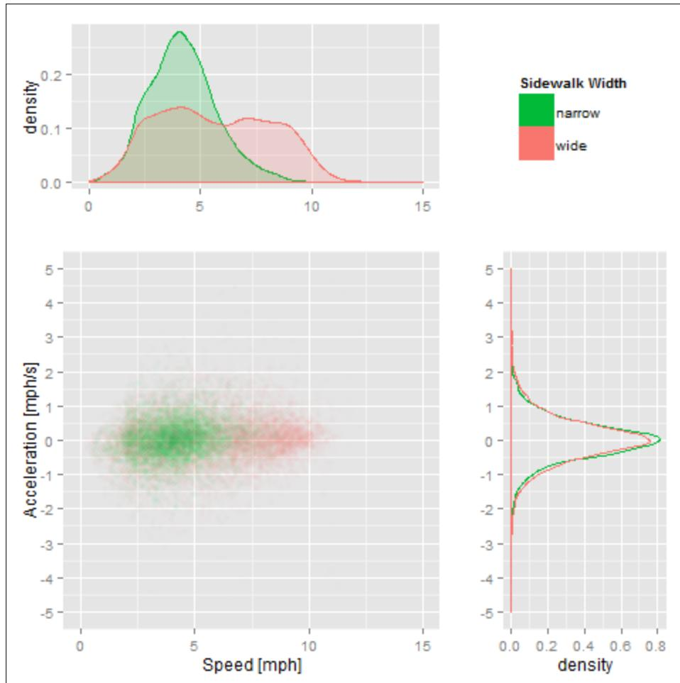
**Figure 50. Segway Test Speed and Acceleration by Sidewalk Width with Heavy Pedestrian Density**
