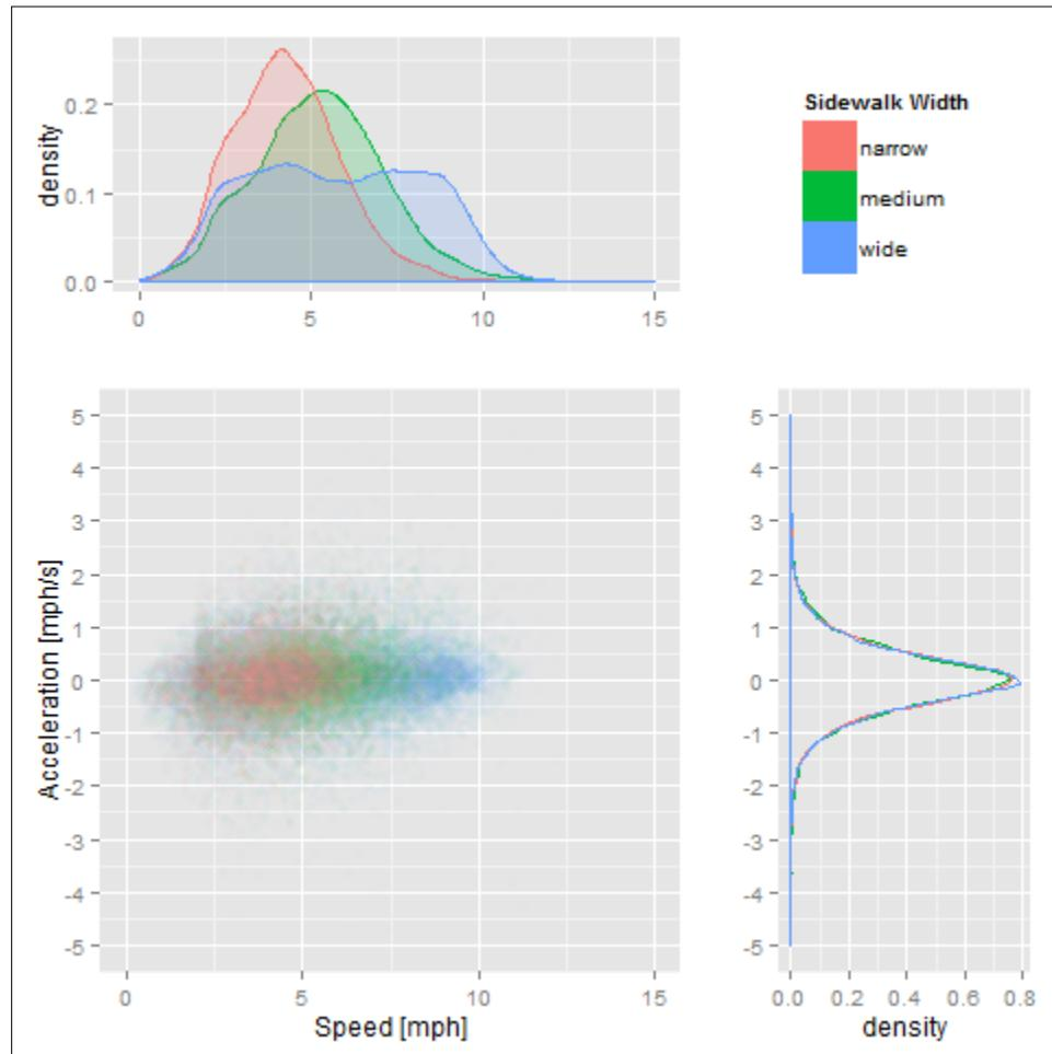
**Figure 43. Effect of Sidewalk Width on Segway Speed and Acceleration**
