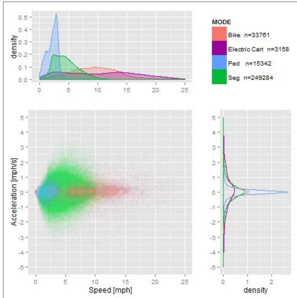
**Figure 40. Modal Comparison of Speed and Acceleration**
