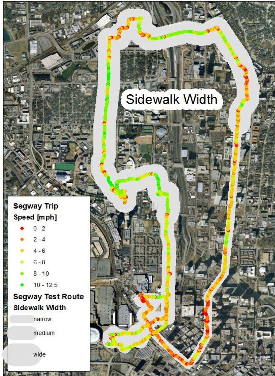
**Figure 42. Map of Segway Test Trip Speed by Sidewalk Width**
