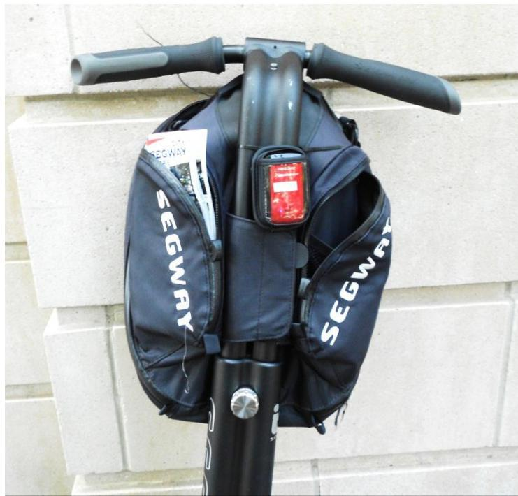
**Figure 32. GPS recorder Instrumented on Segway**
