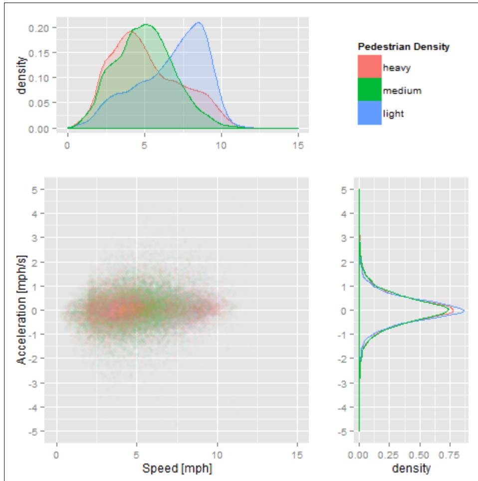
**Figure 47. Effect of Pedestrian Density on Segway Speed and Acceleration**
