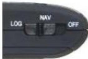
After the completion of each trip, turn the GPS recorder off to conserve battery. Remember to turn it back on prior to beginning your next trip. If you use your personal mobility device(s) very frequently (more than 5 times per day), you may let the device run continually until the battery has been exhausted.
