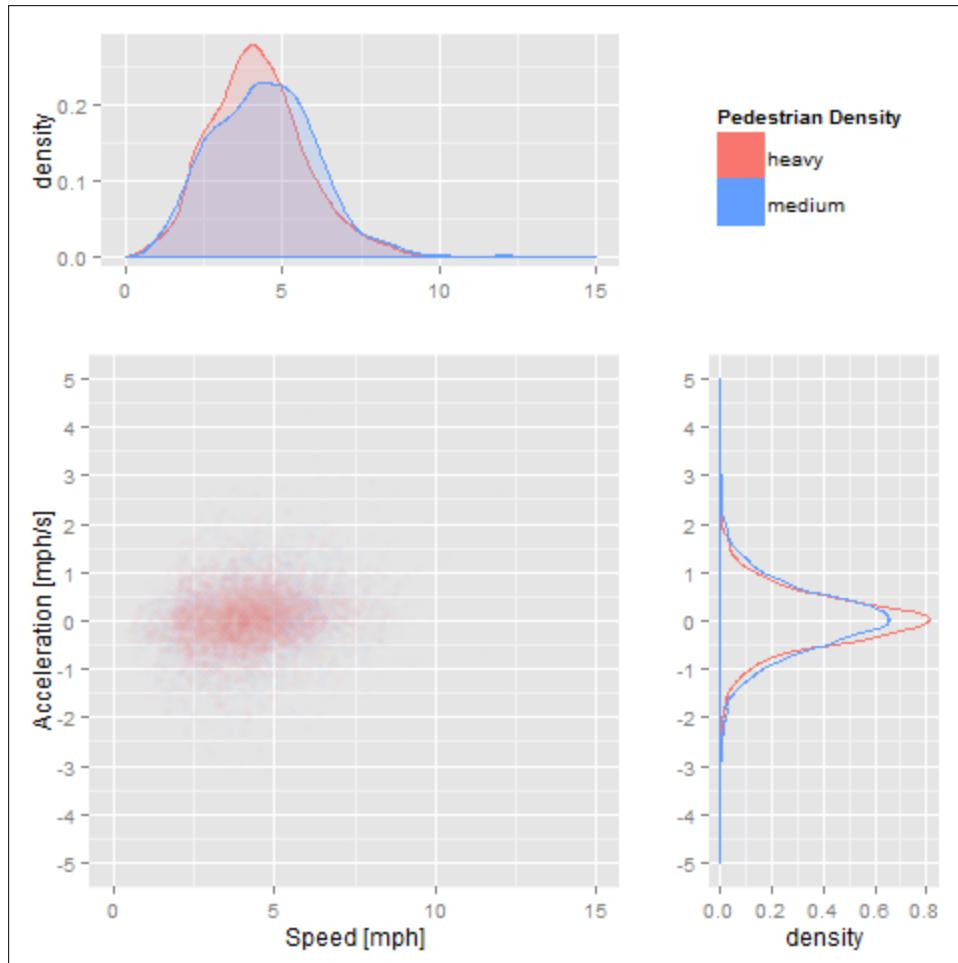
**Figure 49. Segway Test Speed and Acceleration by Pedestrian Density
