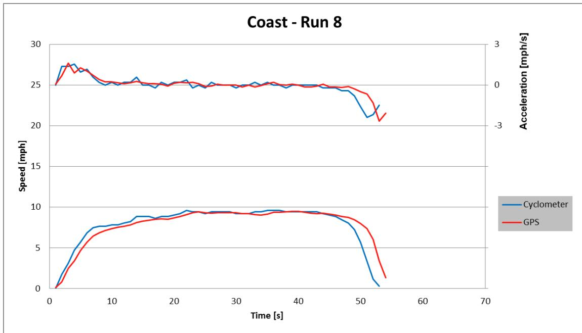
**Figure 74. Lab Test Speed and Acceleration – Coast 8**
